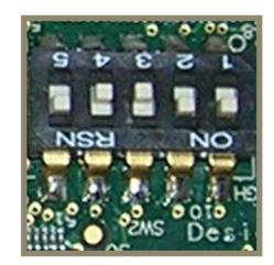
To run Out-Of-Box demo through NAND, configure the switches as shown above.
